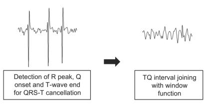
Figure 1 Signal processing diagram to acquire atrial signals without ventricular activities or TQ intervals. A representative TQ interval extracted from ECG by the cancellation of the QRS-T complex was demonstrated.
