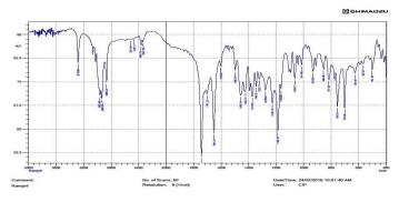
Figure 1: FTIR Spectrum of Ramipril
