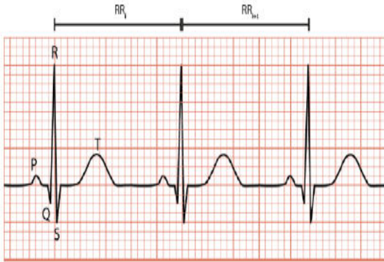
Fig. 4. P Wave, QRS complex, ST wave and T wave representation of ECG signal
