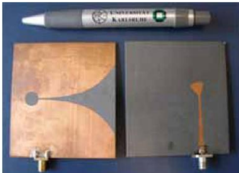
Fig. 6. Aperture coupled Vivaldi antenna. (Left) Top view ;( right) bottom view with feed line. Substrate size 75 _ 78 mm 2 .
