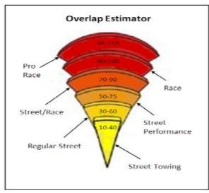
Different amounts of overlap are designed into camshafts depending on the use of the engine. Large amounts of overlap are found in racecars.
