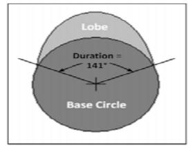
Duration is the amount of time (in degrees) that camshaft lift is generated. In this case, the duration is 141 degrees
