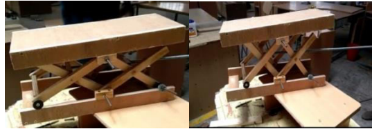
Fig 5.,Prototype of scissor lift constructed initial position (left) and final position (right)
