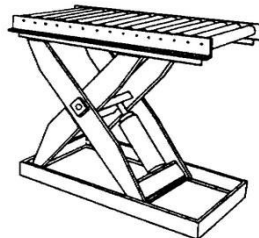
Fig 1.,Scissor Lift Mechanism
