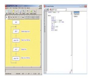
Fig. 3. Program as a flowchart (left) and program in code (right) in Picaxe Programming Editor
