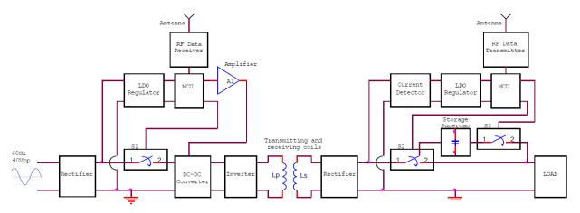
Fig 1: WPT using inductive coupling
