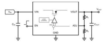
Fig 2: Schematic of a low-dropout regulator
