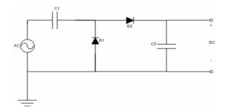
Fig 5: Voltage Doubler Circuit
