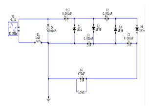
Fig 7: Software Implementation of Receiver Circuit Diagram
