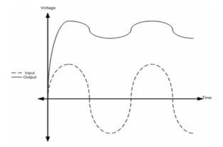
Fig 6: Voltage Doubler Waveform
