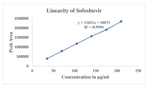
Figure2:Calibrationcurve of Sofosbuvir in therange35to 210 µg/ml.
