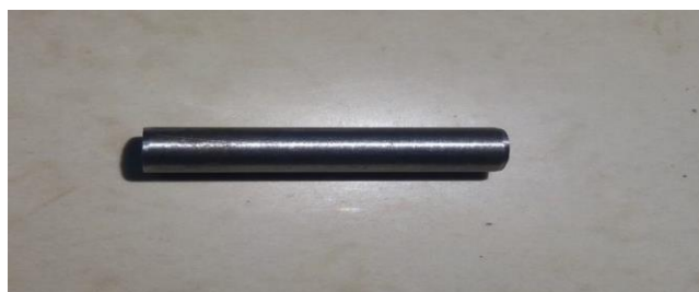
FIG 3.1 SHOWS THE SAMPLE SPECIMEN OF EN-31 STEEL
