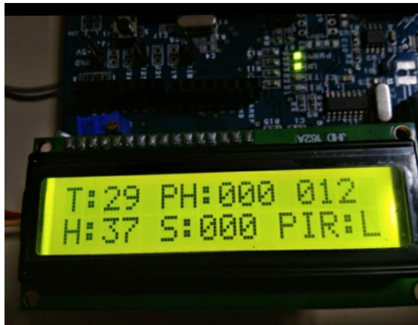
Fig 9 LCD display results of the soil analysis kit
