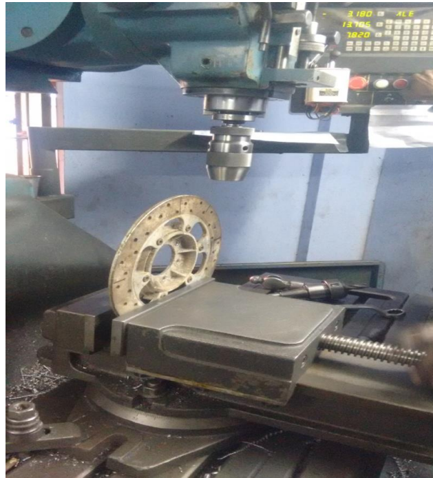
Figure 3 Drilling of Holes in Disc Brake
