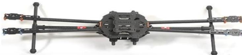
Fig 3: 650 mm Quadcopter Carbon fibre frame
