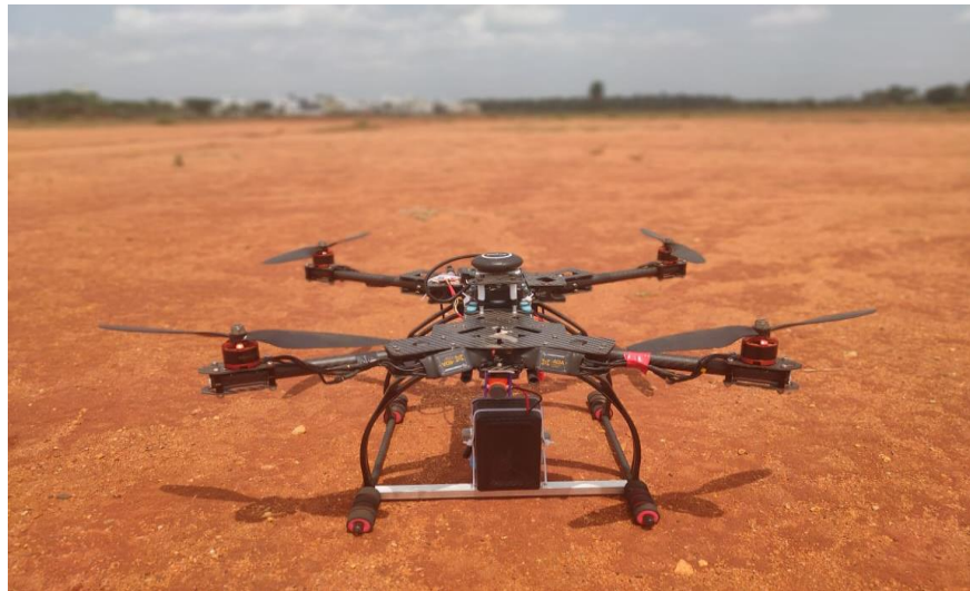
Fig 9: Environmental sensing Quadcopter final prototype
