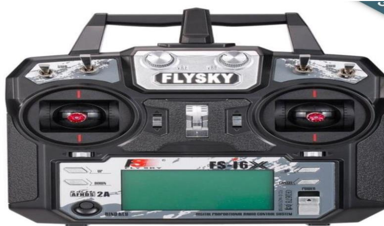
Fig 8: RC Transmitter with FS-IA68 receiver -6CH FLYSKY FS-I6X 2.4GHZ
