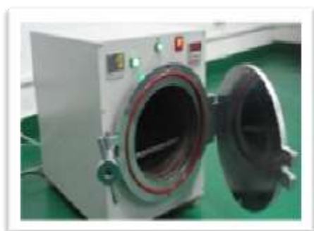
Fig No. 5: Sterilization of Diluted Agar Medium in Autoclave
