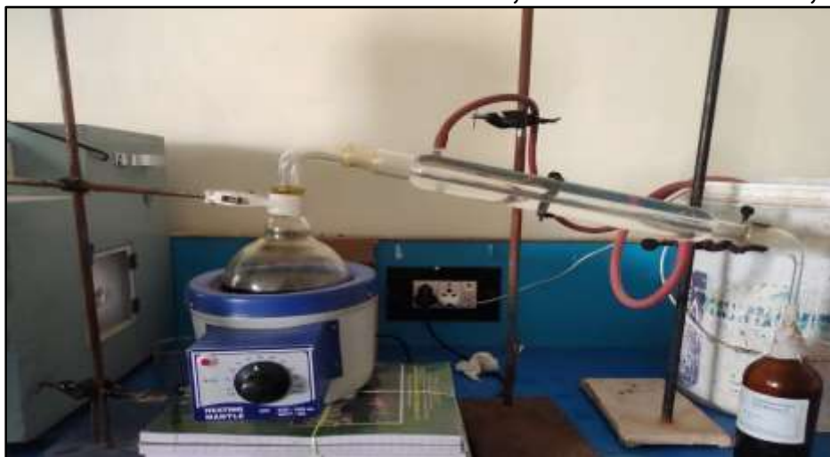
Figure 13: Distillation of crude extract of E. acuminata .
