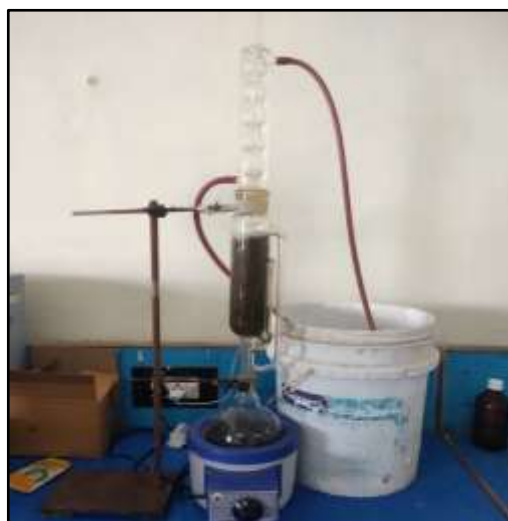
Figure 12: Soxhlet extraction of leaves of E. acuminata .
