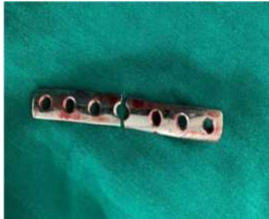
Figure 3: broken clavicle plate after removal
