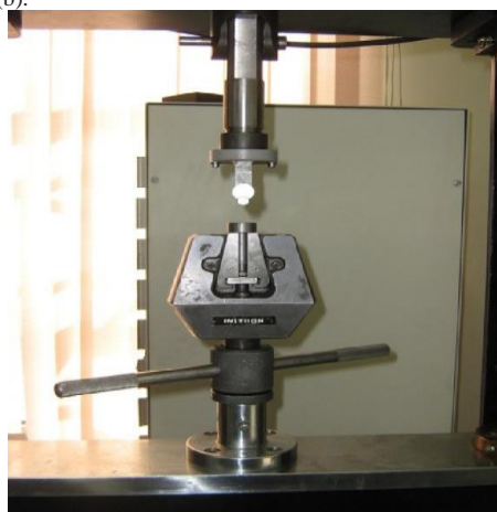
Fig. 4. Universal testing machine (instron) with 5 mm diameter stainless steel ball using for applying load on the alumina cores.
