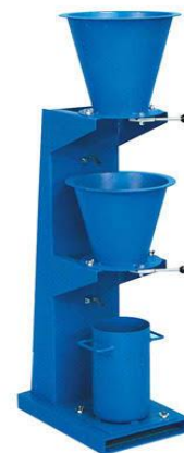
Fig. 1: Compaction factor test.
