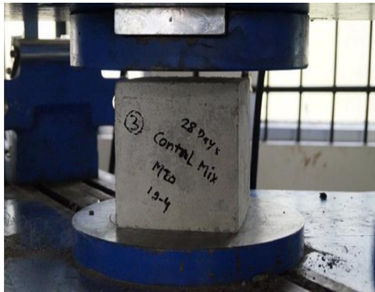
Fig. 2: Compressive strength test of cube samples in CTM.
