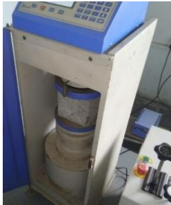
Fig..3.1 Compressive Strength Test of Cubes
