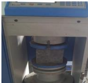
Fig.2.6: Compressive strength testing machine
