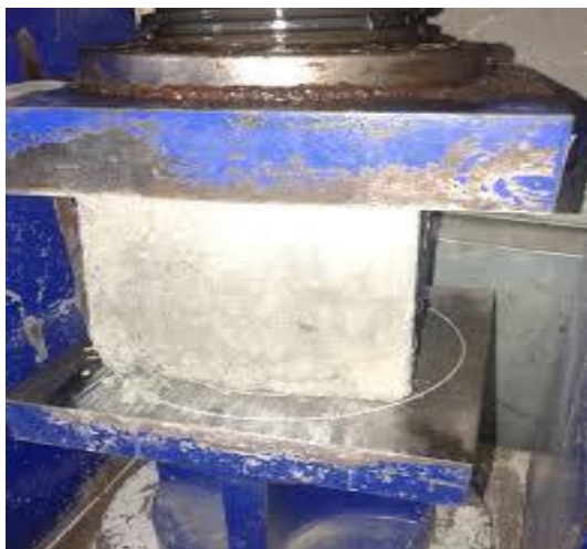
Fig 3.5.1 Compressive strength testing machine
