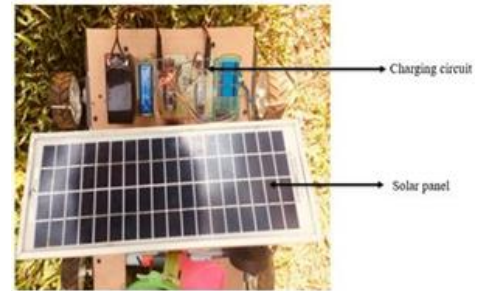
Fig.9. Snapshot of solar charging.
