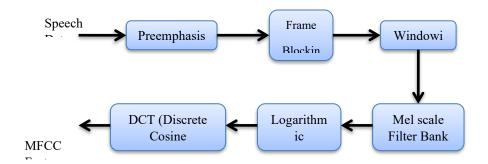
Figure 2: MFCC operation diagram
