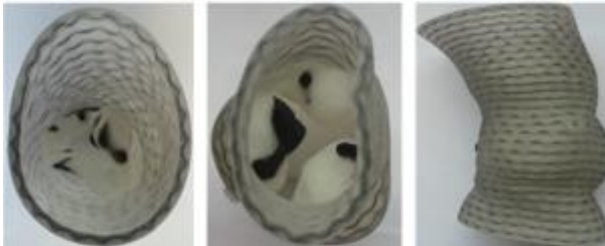
Figure 2: 3D-printed physiological phantoms of an aortic root are shown. The calcifications and the fibers are printed with black materials for better illustration. Image adapted from Wang et al., 2017.
