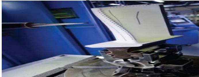
Figure 6: Laser drilling turbine blade
