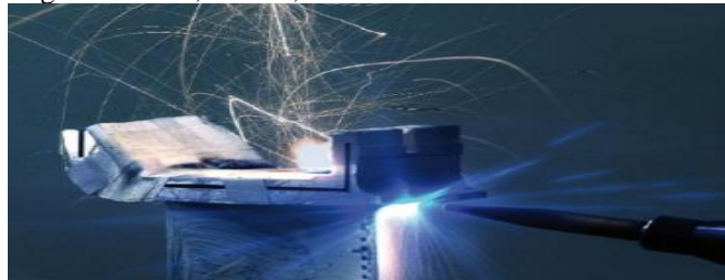
Figure 5: Turbine blade during laser drilling
