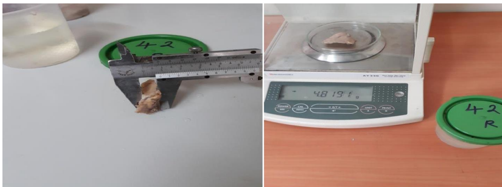
Fig.10.Measurement of Thickness and Weight
