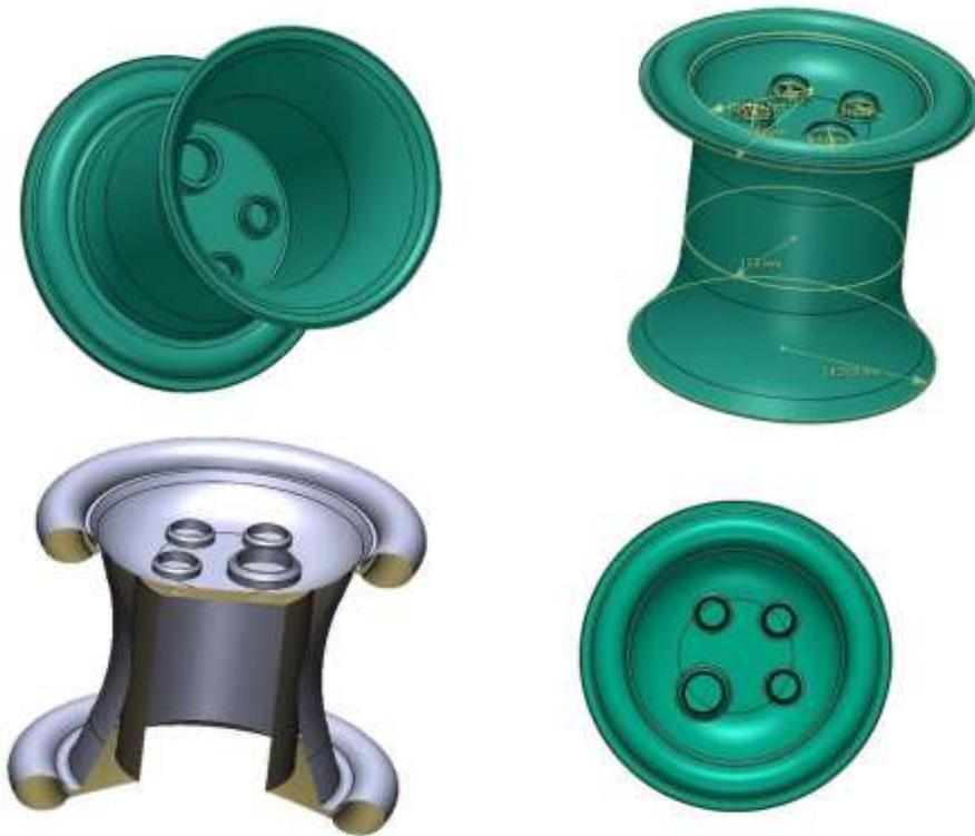
Figure 2: 3D printed SILS port
