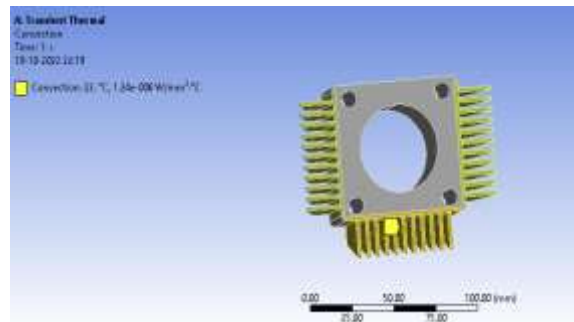
Fig 40: Transient Thermal Convection of Rectangular Fin
