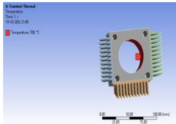
Fig 33: Transient Thermal Temperature of Rectangular Fin
