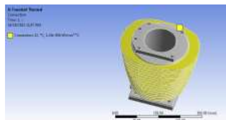
Fig 5: Transient Thermal Temperature of Circular Fin
