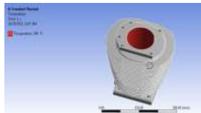
Fig 5: Transient Thermal Temperature of Circular Fin
