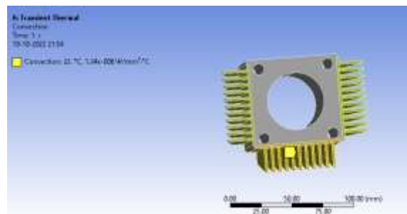
Fig 34: Transient Thermal Convection of Rectangular Fin
