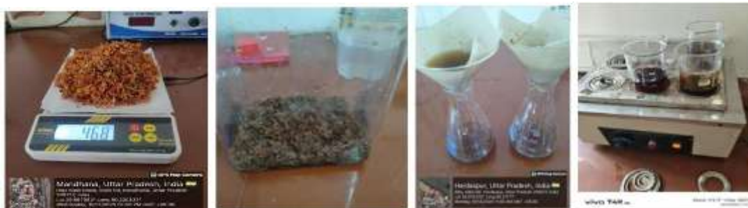
Figure 2: Phytochemical extraction workflow illustrating sequential steps: plant collection and drying, grinding to powder, cold maceration, filtration, and rotary evaporation
