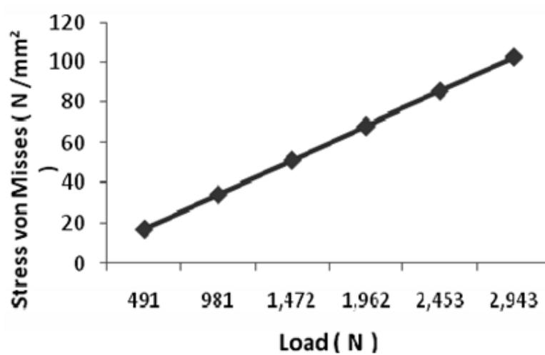
Figure 4: Load versus Von Misses stress
