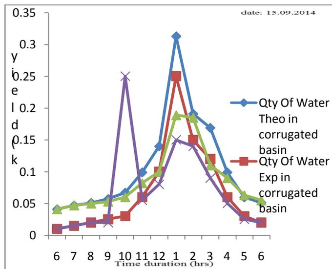
Figure 5 : Hourly variations of Experimental & Theoretical Yield.in single slope solar still
