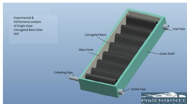
Fig1. Diagram of single slope single corrugated basin.
