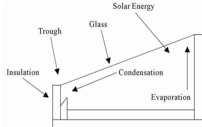
Fig 2. Model diagram for simple single slope single basin solar still
