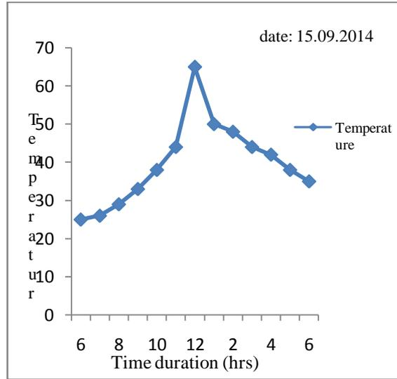
Figure 3: Hourly variation of basin water temperature for a day of experiment in corrugated basin
