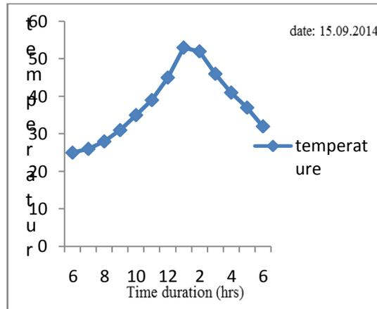
Figure 4 :Hourly variation of basin water temperature for a day of experiment in normal basin
