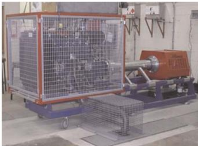
Figure 1. Experimental set-up of Kubota V3300 Indirect Injection, four cylinders naturally aspirated CI engine
