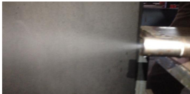
Fig 11. Atomization of fuel at 2 bar pressure
