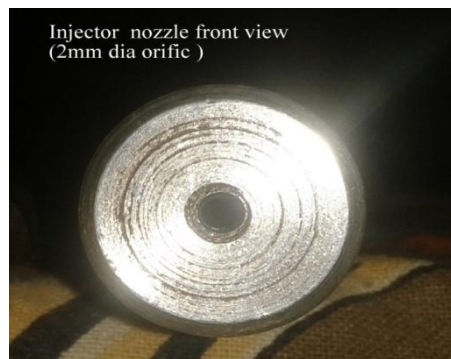
Fig 7. Injector nozzle with 2mm diameter
