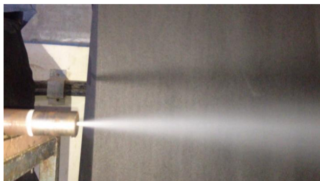
Fig 12. penetration length increased at 4 bar pressure
