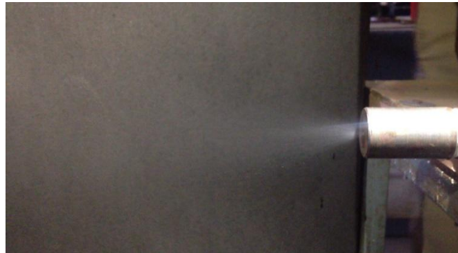
Fig 13. Spray cone angle increased at 3 bar pressure
