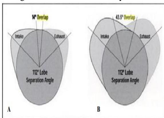
Overlap is the amount of time (in degrees) that both the intake and exhaust valves are open. Camshaft B has more duration than Camshaft A, causing an additional overlap, 43.5 degrees versus 14 degrees, in order to maintain the same LSA
