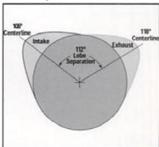
Centerline is the term used to determine the placement of the lobes both on the camshaft and in the engine. The camshaft profile shown has an intake centerline of 106 degrees and an exhaust centerline of 118 degrees
