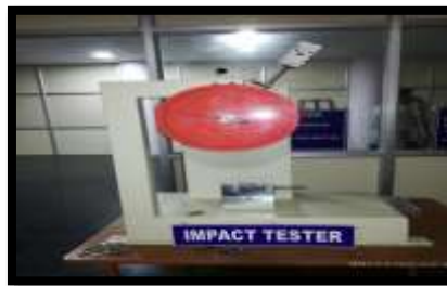
Figure 22 Impact machine for impact testing
