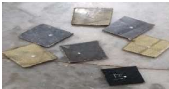
Figure 28 AFTER TESTING OF HARDNESS SPECIMENS
