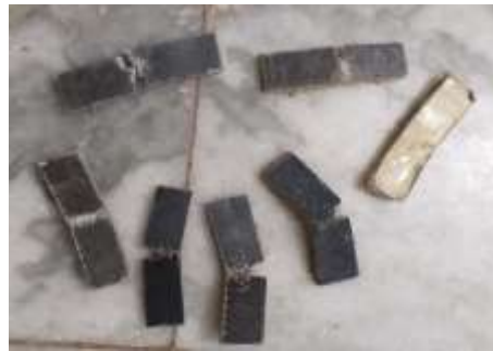
Figure 27 AFTER TESTING OF IMPACT SPECIMENS
