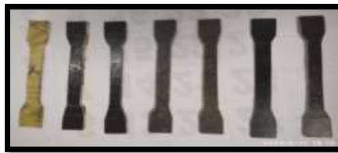
Figure 20 Tensile test specimens
